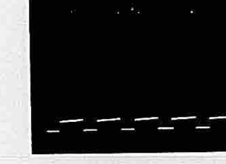
29 U318, Pin 15 SEGMENT SELECT 1b X10 Probe DC Coupled Internal Negative Sync
