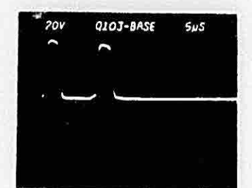
6 Q103, base Q103 MODULATOR BASE DRIVE X10 Probe AC Coupled Internal Positive Sync
