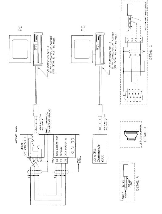
FIGURE 2-18 KLN 90B DATALOADER/PC INTERFACE DRAWING
