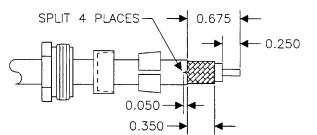
Place cable nut, bushing and braid clamp over outer jacket. Trim cable jacket, braid and dielectric to dimensions shown. Split outer jacket in 4 places (approx. 90° apart) to dimension. Lightly tin center conductor.
