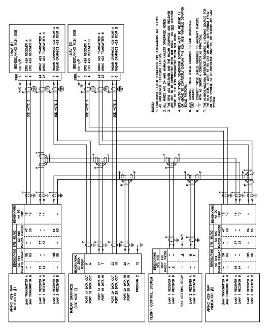
FIGURE 2-17 KLN 90B INTERCONNECT DRAWING (DWG NO. 155-06021-0000, R-AC) (SHEET 1 OF 10)
