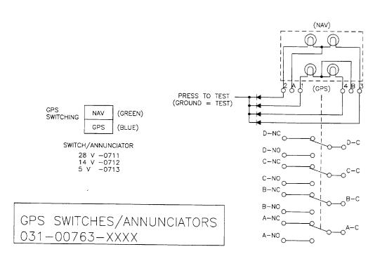
FIGURE 2-16 CUTLER-HAMMER SWITCH/ANNUNCIATOR INTERNAL SCHEMATIC (SHEET 1 OF 2)
