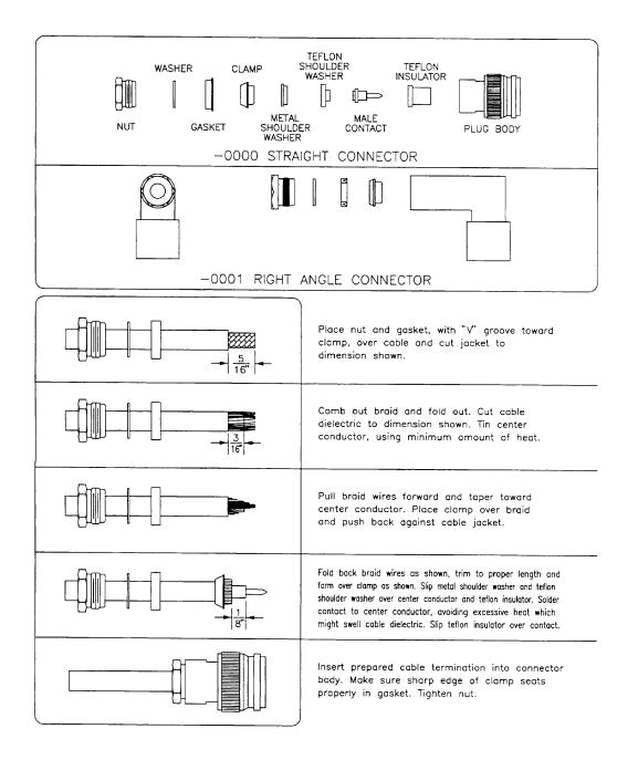
FIGURE 2-10 KA 91/92 TNC ANTENNA COAX/CONNECTOR ASSEMBLY RG142B/U OR RG400 0 TO 40 FT. (P/N 030-00134-0000, R-3 / 030-00134-0001, R-0)
