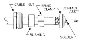
Slide contact assembly (pin or socket) between inner dielectric and foil shield. Make certain contact assembly is pushed on cable to flare outer jacket and center conductor is visible through inspection hole. Smooth shields back over contact assembly and solder center contact as shown.
